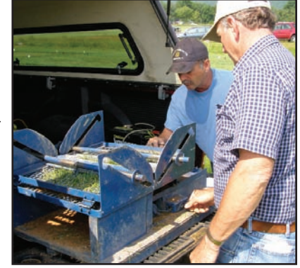
Once the sod is plated and locked down, it is stretched until it tears and the pounds at which it separates is recorded.
